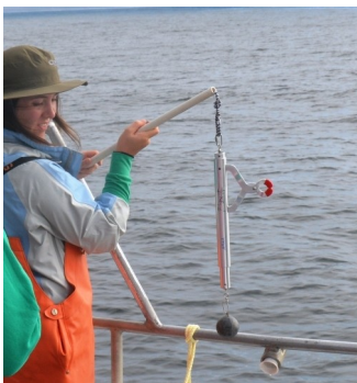
The Blacktip Catch and Release Recompression Tool can be rigged on a rod or a rope and needs a weight. Cost is $35.00
