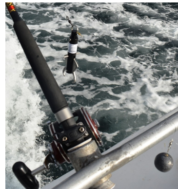
The SeaQualizer can be programmed to automatically release at 50, 100, or 150 feet. Cost is $50.00 plus weight
