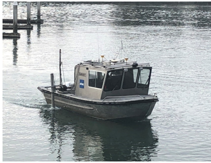
Survey boat that maps depths before dredging to determine where material needs to be removed and after dredging to ensure target depths are reached.
